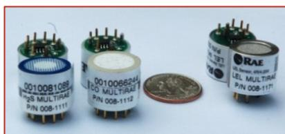
reaction that changes the electrical balance in the sensor. The poles detect the change which results in a reading. However, one of the challenges in detecting toxic gases is how precise the sensor is in detecting the target gas. The carbon monoxide sensor will react to quite a few other gases, some of which are listed in Table 2.
