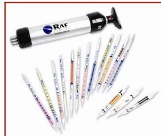
It will then take one to three minutes for the air sample to be drawn into the tube. When using the bellows-style pump you squeeze, release, and wait for the bellows to expand fully before squeezing again. This method requires the user to track the number of pumps it takes to draw the proper amount of air through the tube. Most sample pumps and piston pumps have an indicating mechanism that alerts the user that the pump stroke is complete.
