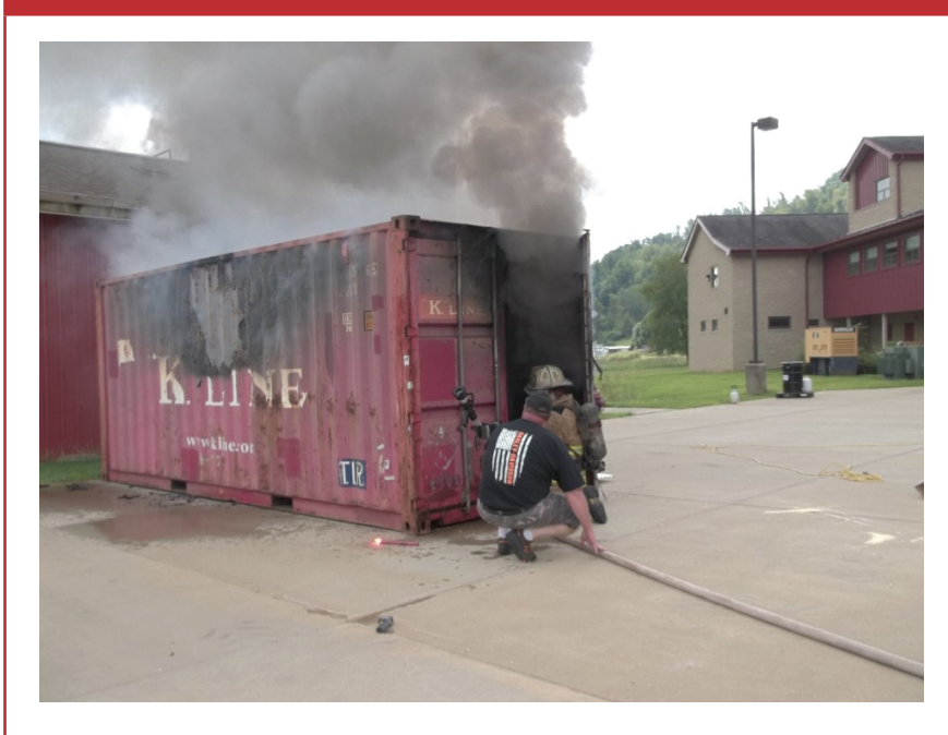
Figure 4: Fire load materials after burn in metal shipping container
