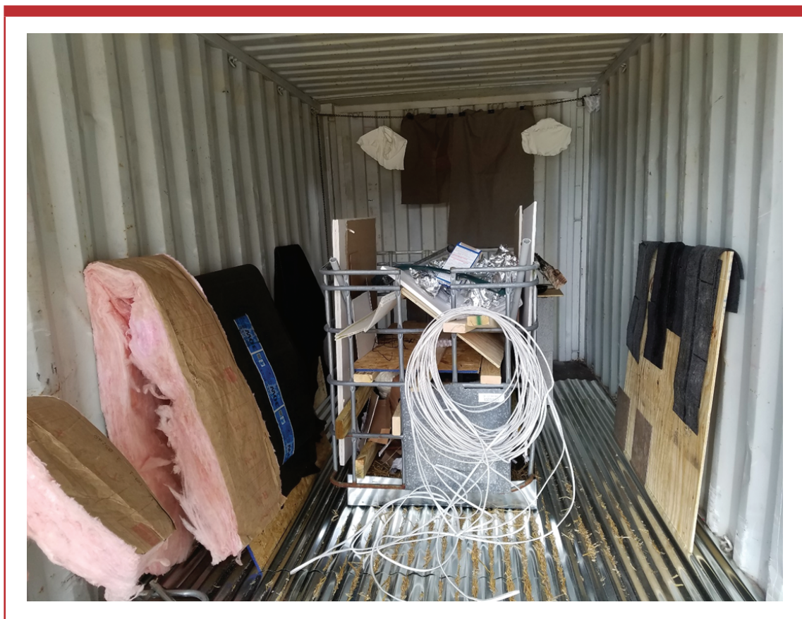
Figure 2: Layout of fire load materials inside metal shipping container (fabric panels are seen at back of box covering ventilation hole)
