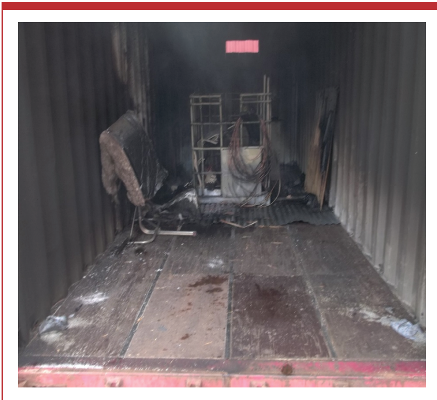
Figure 4: Fire load materials after burn in metal shipping container
