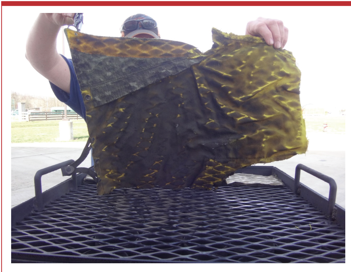
Figure 10: Inconsistent smoke deposits on sample material after MCC burn
