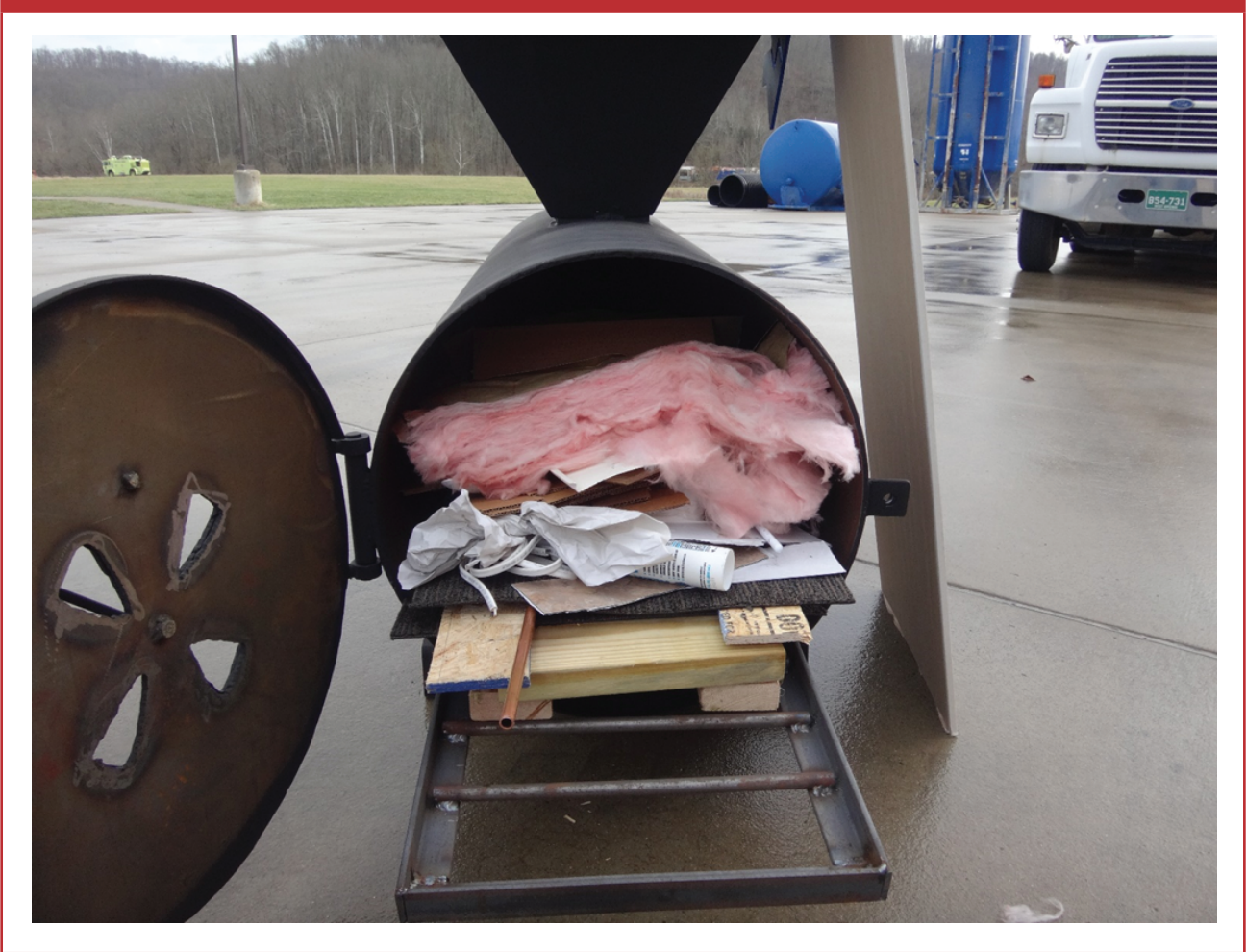
Figure 8: Layout of fire load materials inside MCC
