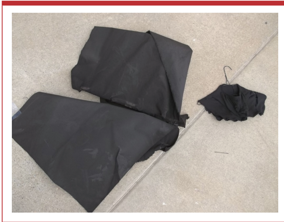
Figure 5: Deteriorated fabric samples affected by extensive heat in large scale burn
