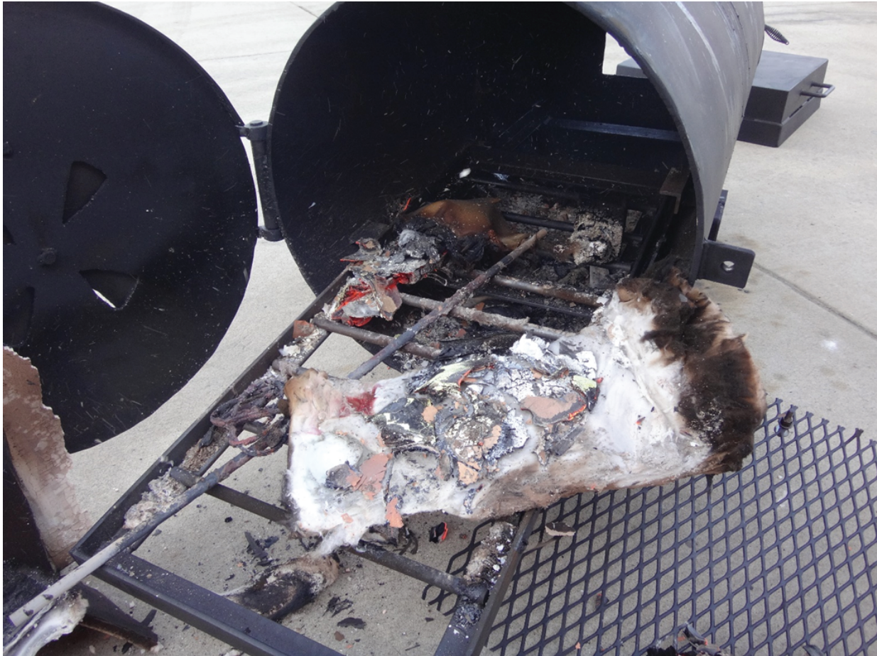
Figure 9: Fire load materials after burn in MCC
