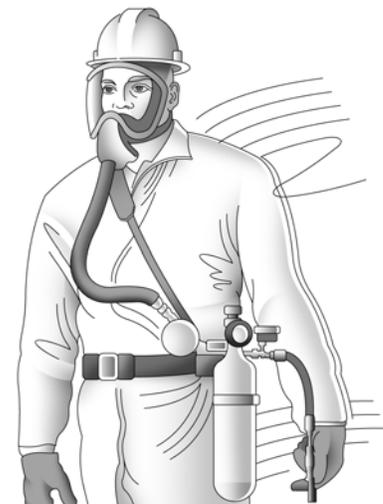
**Tight-fitting Atmosphere-Supplying Respirator with an auxiliary escape bottle**
