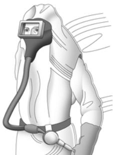
**Abrasive Blasting Respirator; Atmosphere-supplying respirator Full Facepiece Elastomeric**
