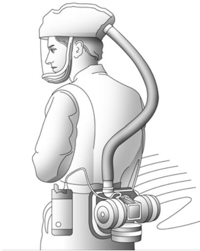
**Loose-Fitting Powered Air-Purifying Respirator (PAPR)**
