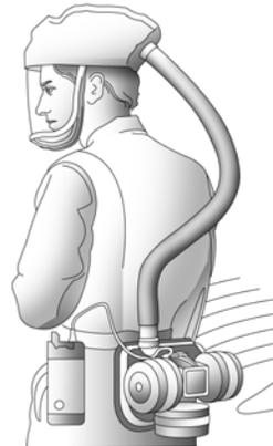
**Loose-Fitting Powered Air-Purifying Respirator (PAPR)**
