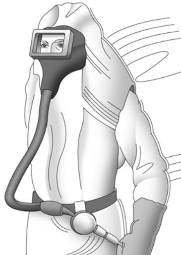
**Tight-fitting Abrasive Blasting Respirator Continuous flow**
