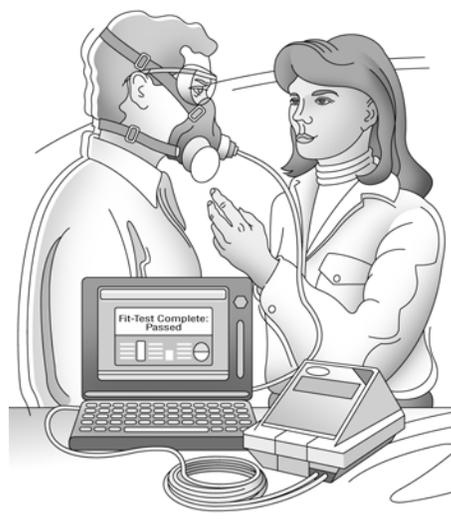
**Quantitative fit testing.** To conduct quantitative fit testing on an atmosphere-supplying respirator, you must temporarily or permanently install a sampling probe or adaptor inside the facepiece.
