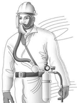
**Atmosphere-supplied respirator Full Facepiece Elastomeric with an auxiliary escape bottle**
