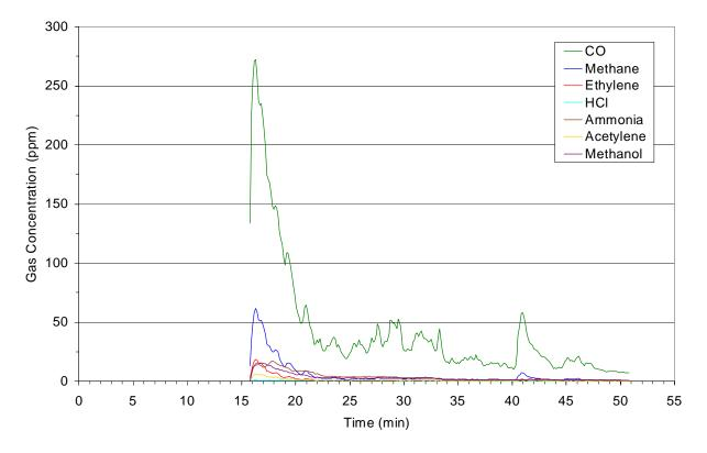
**Figure 4-42: Gas concentration measured by extractive FTIR during overhaul of the kitchen fire.** Peak gas concentrations and calculated total exposures are summarized in Table 4-17.
