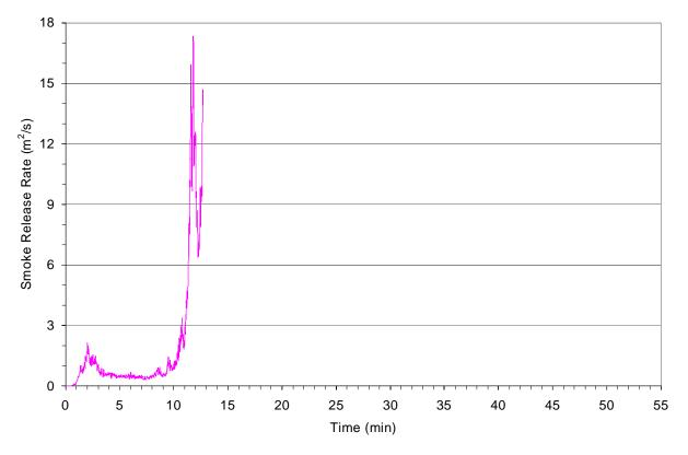
Figure 4-56: Smoke release rate during the fire growth phase of the wood deck fire.
