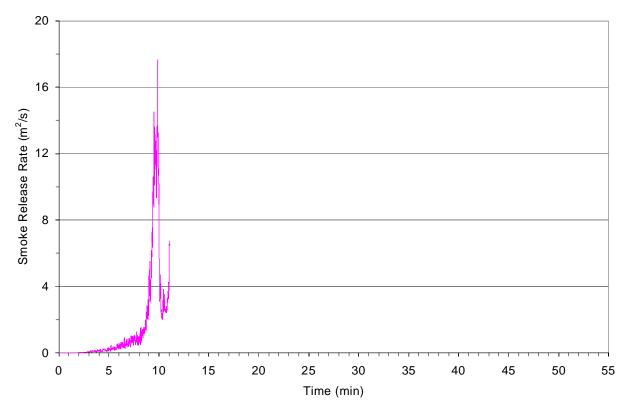
Figure 4-41: Smoke release rate during the fire growth phase of the kitchen fire.
