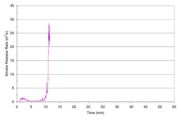
Figure 4-64: Smoke release rate during the fire growth phase of the composite deck fire.
