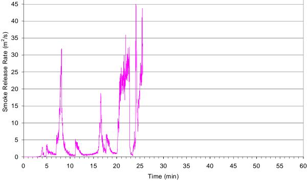
Figure 4-25: Smoke release rate during the fire growth phase of the limited ventilation living room fire.
