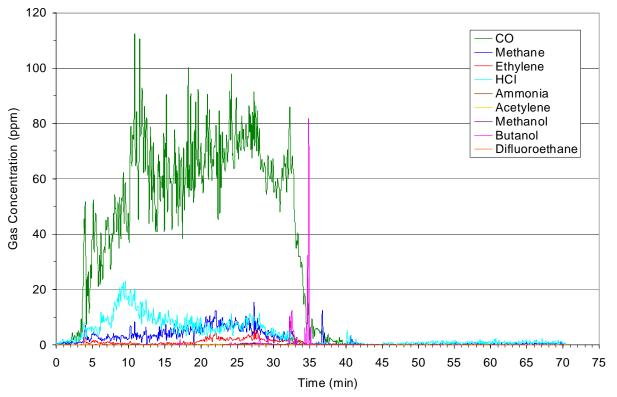
**Figure 4-73: Gas concentration measured by OP-FTIR for the passenger compartment fire.** Peak gas concentrations and calculated total exposures are summarized in Table 4-40.
