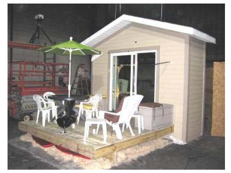
Figure 4-8: Photograph showing the wood deck scenario with furnishings. Note the the gas and particle sampling probe extending from the right of the sliding glass door over the deck at standing face level.
