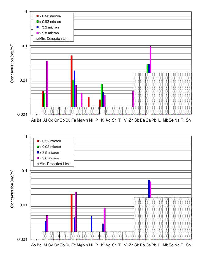
Figure 4-62: Inorganic element concentrations measured for smoke particles collected with personal cascade impactors during overhaul of the wood deck fire.
