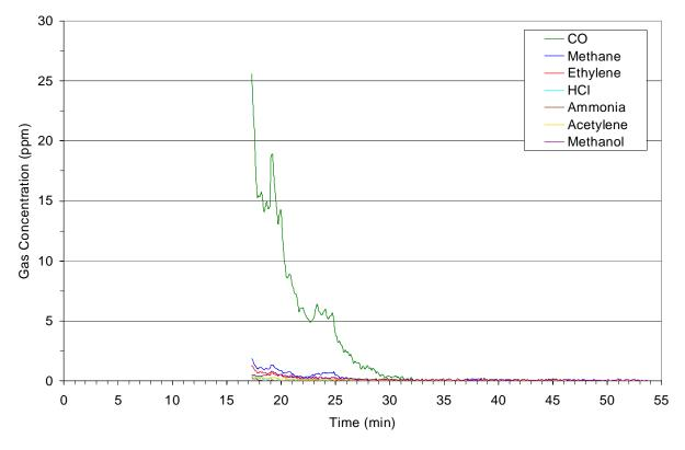
**Figure 4-66: Gas concentration measured by extractive FTIR during overhaul of the composite deck fire.** Peak gas concentrations and calculated total exposures are summarized in Table 4-35.
