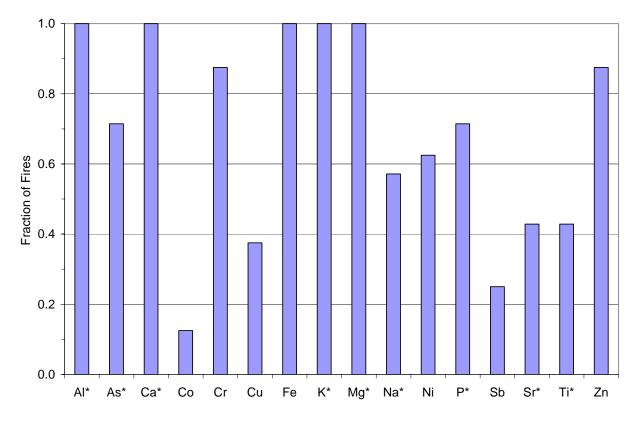
Figure 4-95: Frequency of large-scale fires in which inorganic elements were detected in personal impactor collected smoke particles.
