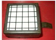
Figure 3-3: ASTM E1354 Cone calorimeter sample holder
