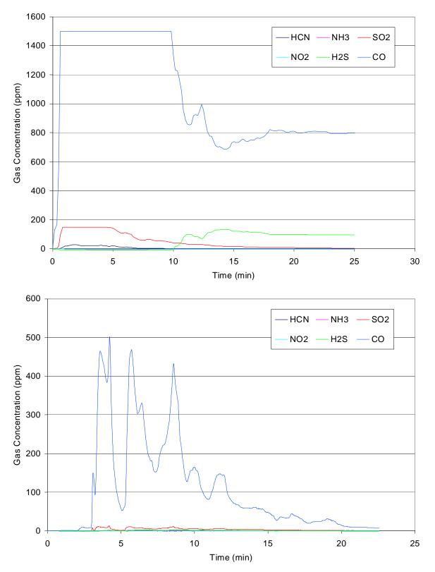
Figure 6-1: Examples of personal gas monitor data. Note how the carbon monoxide and sulfur dioxide sensors saturated during the fire presented in the top figure.
