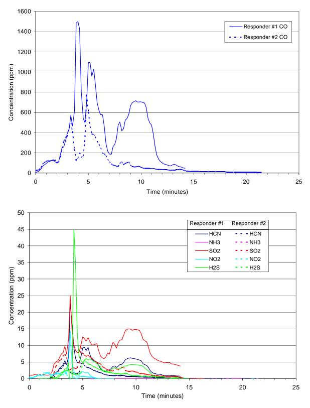
Figure 5-11: Gas concentrations measured by personal monitors for the kitchen fire.
