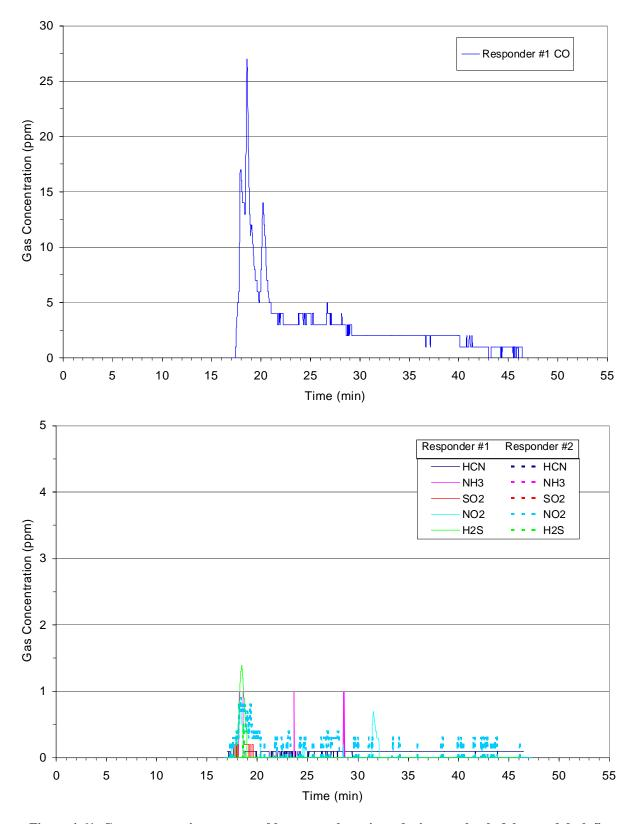
Figure 4-61: Gas concentrations measured by personal monitors during overhaul of the wood deck fire.
