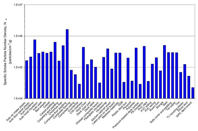
Figure 3-8: Specific smoke particle number density N<sub>m</sub> for material-level test samples.
