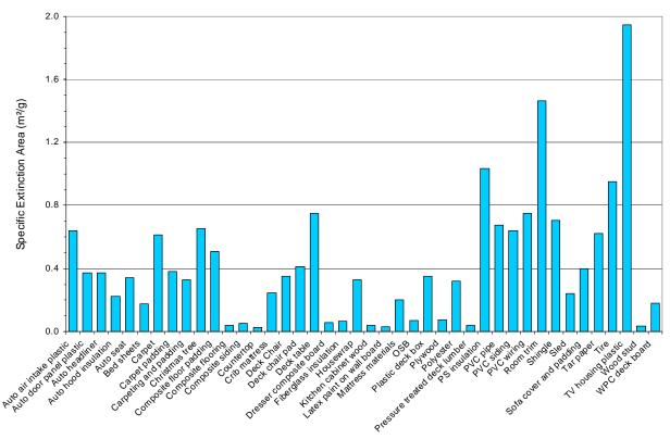
Figure 3-6: Smoke production for material-level test samples.
