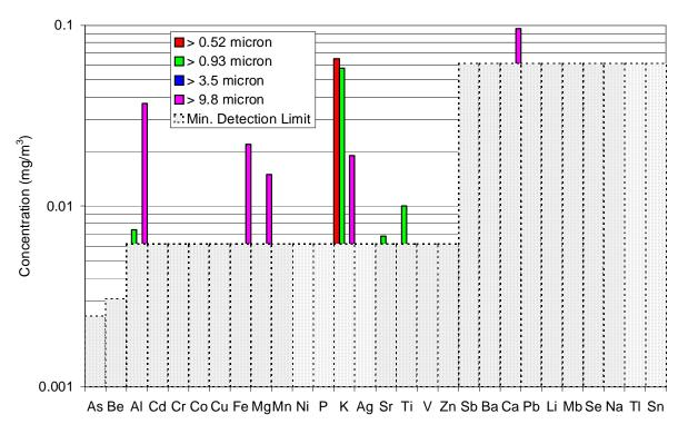
Figure 5-12: Inorganic element concentrations measured for smoke particles collected using personal cascade impactor for the kitchen fire.
