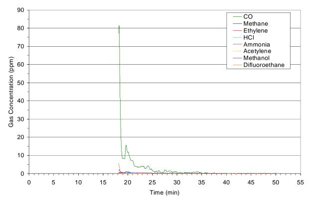
**Figure 4-58: Gas concentration measured by extractive FTIR during overhaul of the wood deck fire.** Peak gas concentrations and calculated total exposures are summarized in Table 4-29.
