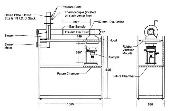
Figure 3-2: Schematic of ASTM E 1354 cone calorimeter (reprinted from ASTM E 1354).
