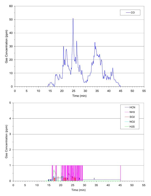
Figure 4-53: Gas concentrations measured by personal monitors during overhaul of the attic fire.
