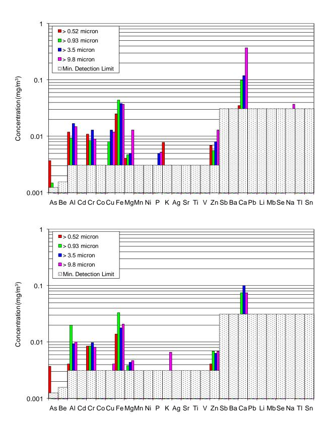
Figure 4-70: Inorganic element concentrations measured for smoke particles collected with personal cascade impactors during overhaul of the composite deck fire.
