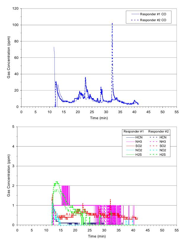
Figure 4-22: Gas concentrations measured by personal monitors during overhaul of the living room fire.
