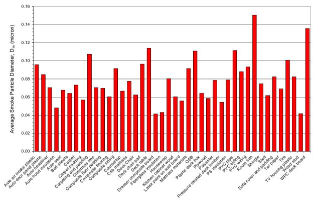
Figure 3-7: Average smoke particle diameter D<sub>m</sub> for material-level test samples.
