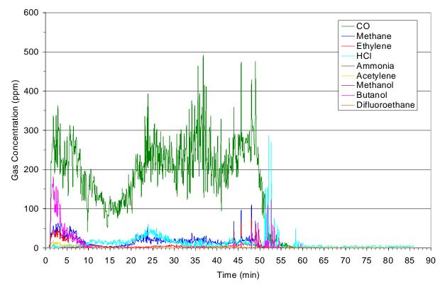
Figure 4-80: Gas concentration measured by OP-FTIR for the engine compartment fire.
