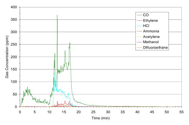
Figure 4-57: Gas concentration measured by OP-FTIR for the wood deck fire.
