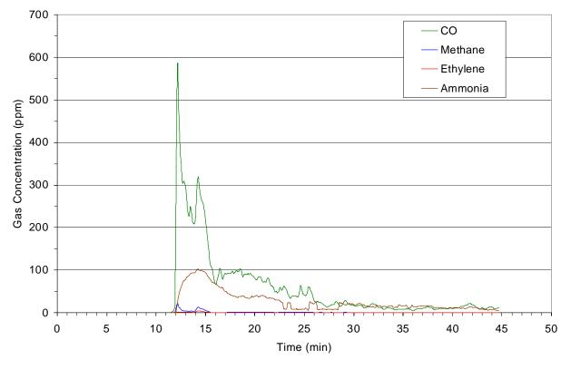
**Figure 4-35: Gas concentration measured by extractive FTIR during overhaul of the bedroom fire.** Peak gas concentrations and calculated total exposures are summarized in Table 4-13.
