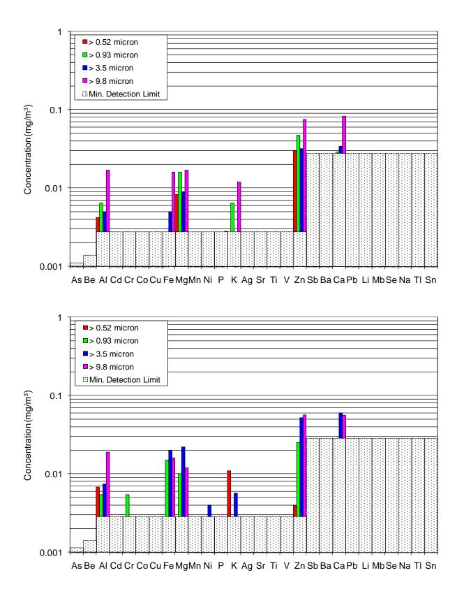
Figure 4-85: Inorganic element concentrations measured for smoke particles collected with personal cascade impactors during overhaul of the engine compartment fire.
