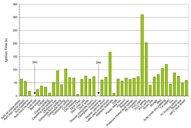
Figure 3-4: Time to ignition for material-level test samples.
