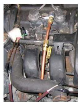
Figure 4-15: Automobile engine compartment fire initiation device.
