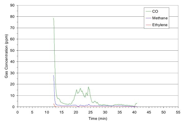
Figure 4-19: Gas concentration measured by extractive FTIR during overhaul of the living room fire. Peak gas concentrations and calculated total exposures are summarized in Table 4-2.
