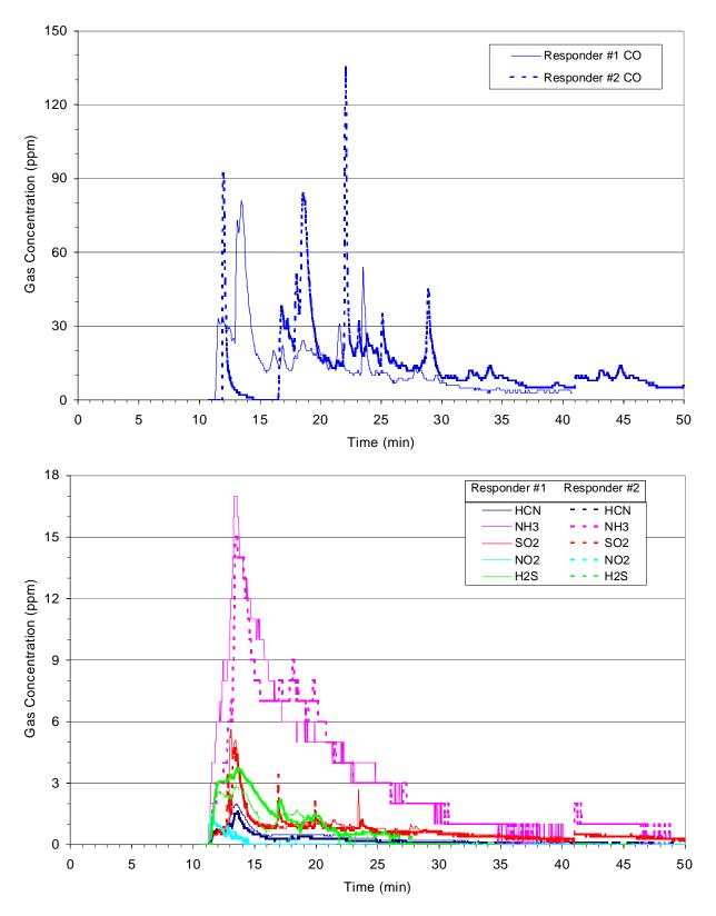
Figure 4-38: Gas concentrations measured by personal monitors during overhaul of the bedroom fire.
