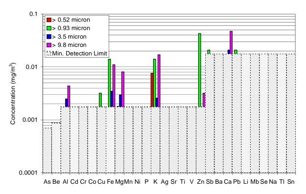
Figure 5-8: Inorganic element concentrations measured for smoke particles collected using personal cascade impactor for the study/small bedroom fire followed by the bathroom fire.
