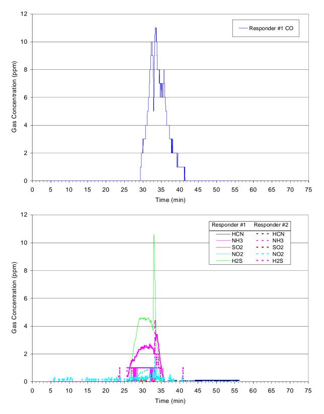
Figure 4-77: Gas concentrations measured by personal monitors during overhaul of the passenger compartment fire.
