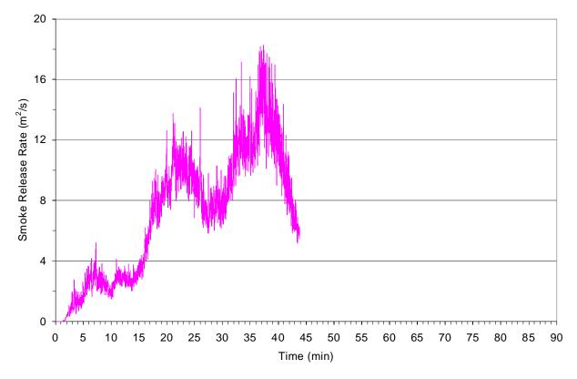
Figure 4-79: Smoke release rate during the fire growth phase of the engine compartment fire.
