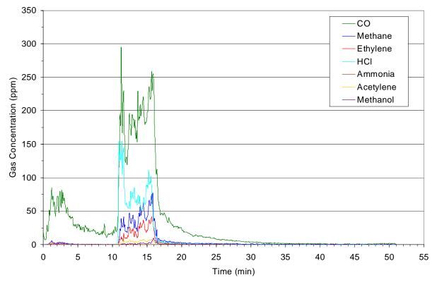
Figure 4-65: Gas concentration measured by OP-FTIR for the composite deck fire.
