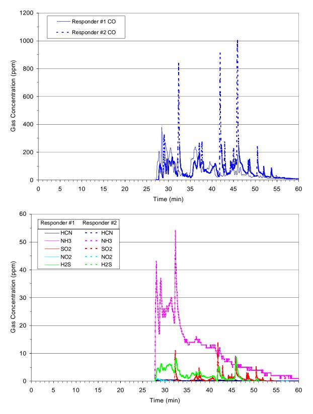
Figure 4-30: Gas concentrations measured by personal monitors during overhaul of the limited ventilation living room fire.
