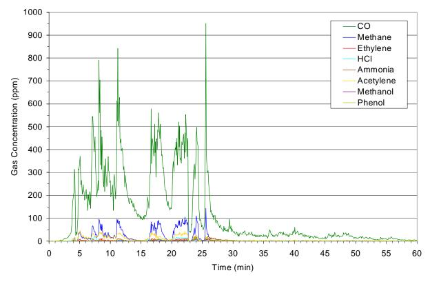
**Figure 4-26: Gas concentration measured by OP-FTIR for the limited ventilation living room fire.** Peak gas concentrations and calculated total exposures are summarized in Table 4-6.
