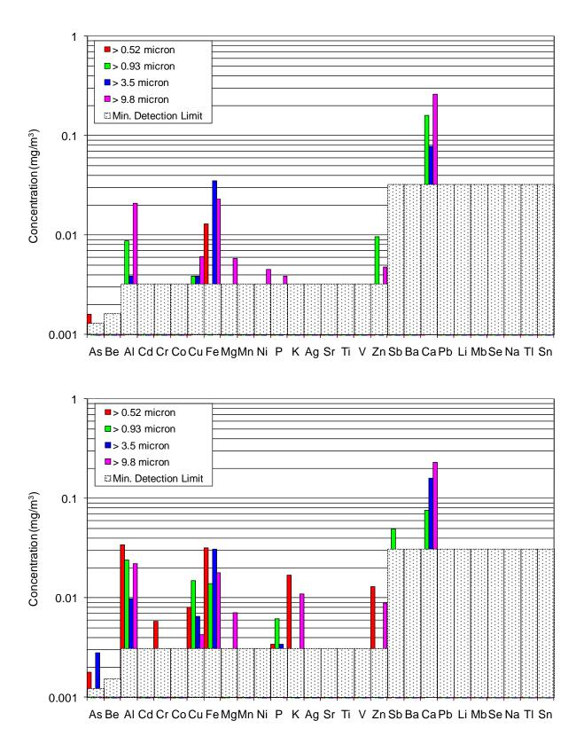
Figure 4-54: Inorganic element concentrations measured for smoke particles collected with personal cascade impactors during overhaul of the attic fire.
