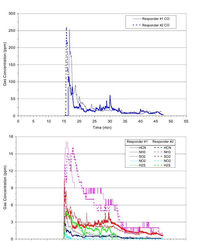
Figure 4-45: Gas concentrations measured by personal monitors during overhaul of the kitchen fire.
