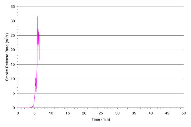
Figure 4-33: Smoke release rate during the fire growth phase of the bedroom fire.
