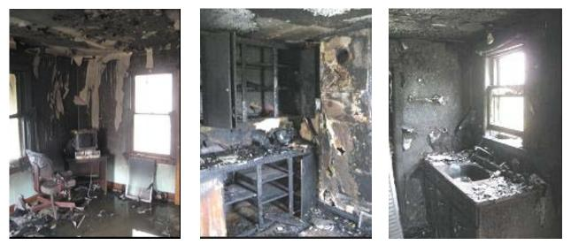
Figure 5-10: Kitchen after the controlled field fire event.
