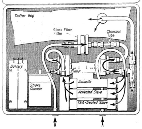
Figure 1 - Principal components of air sampler.
