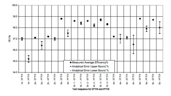
Figure 5-12. Calculated Combustion Efficiencies with Uncertainty Bars for EFTIR and PFTIR
