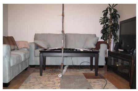
Figure 4-3: Photograph of the furnished living room interior for the limited ventilation fire test. Note the thermocouple instrumented post in the center of the room.
