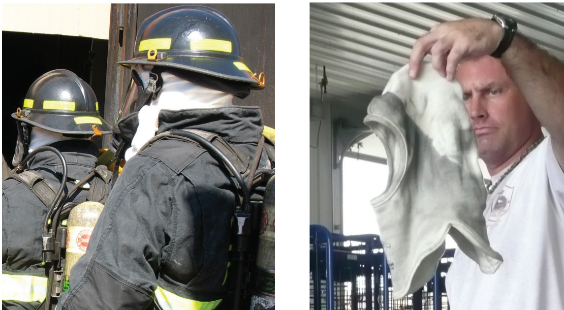
Figure 26. (Left) Photograph of fire fighter in full ensemble showing the area of the neck that is protected primarily by the white Nomex hood; (Right) Hood after being worn once for a fire suppression exercise during round 1. Photos by NIOSH.
