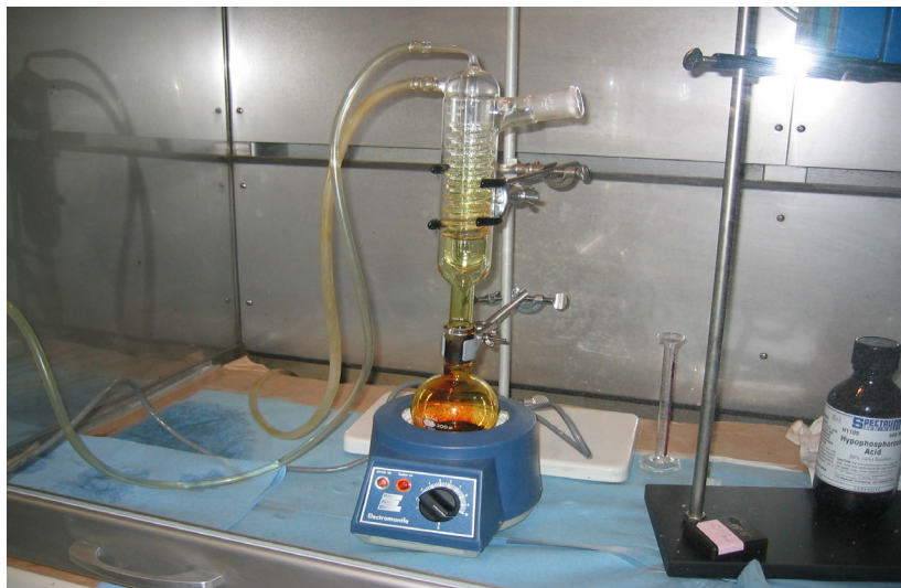
Figure 1: Iodine staining on condenser tube in laboratory hood.
