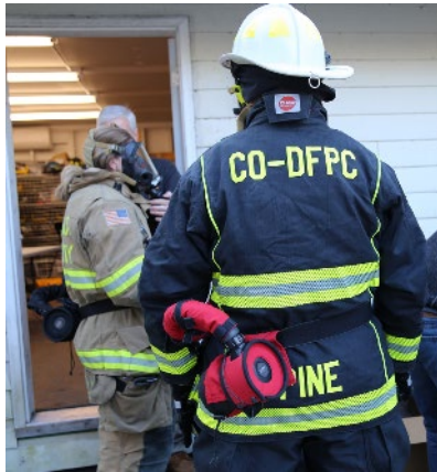
Figure 1-3 EZ-Air PAPR with Single Filter
