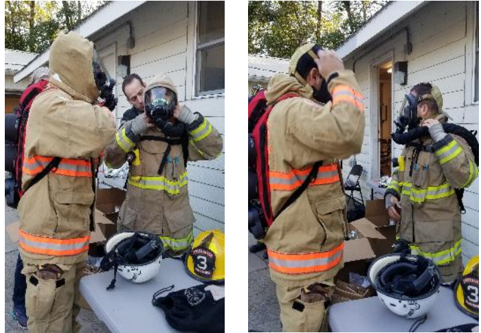
Figure 3-3 Evaluators are Fitted with the MP-PAPR Filter System
