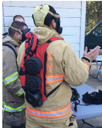
Figure 1-4 MP-PAPR with Two Filters
