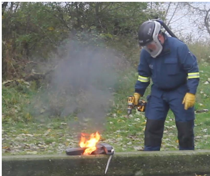
Figure 1 - Lithium battery test burn while wearing proper PPE, including a powered air purifying respirator. Credit: Dr. Peter Mansi.
