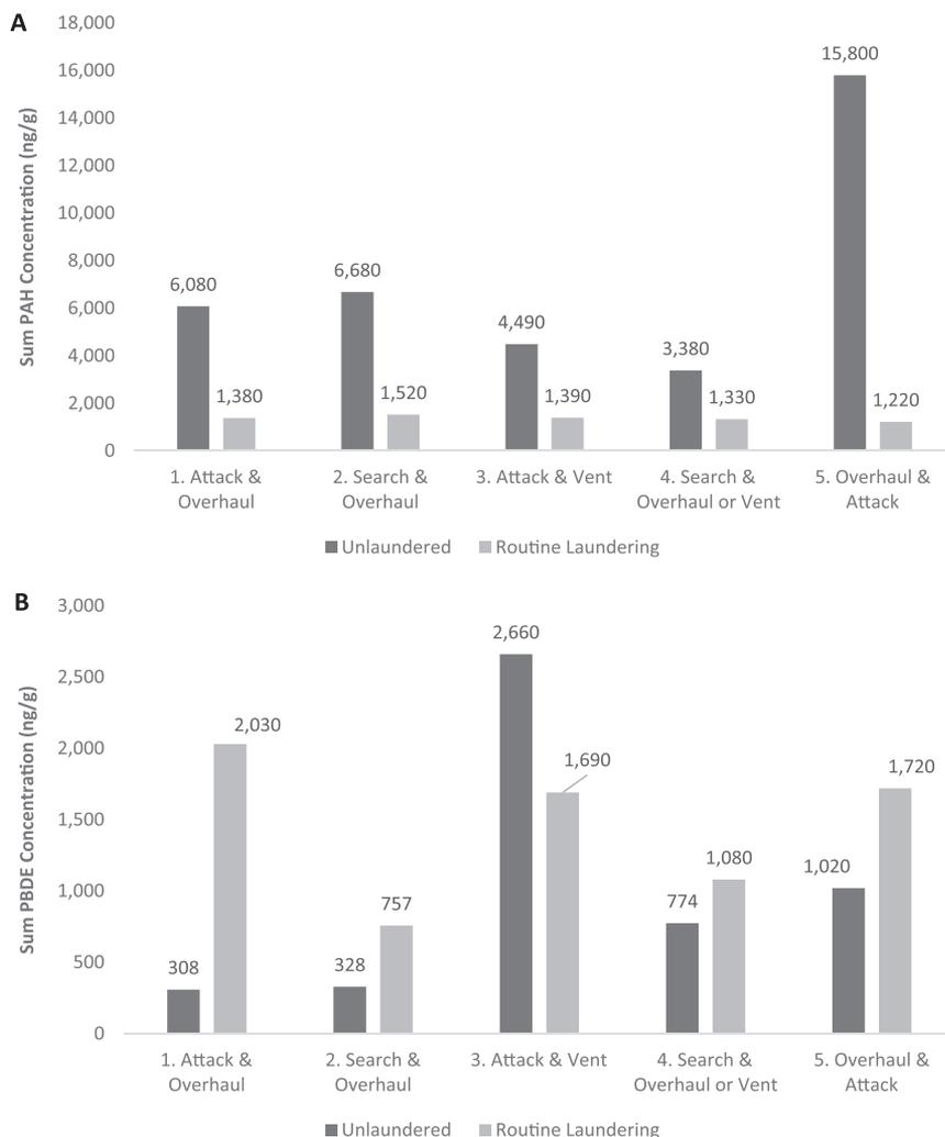
**Figure 1.** Total levels of (A) PAHs, (B) PBDEs, (C) NPBFs, and (D) OPFRs measured in hoods routinely laundered or unlaundered after a total of four fire scenarios by job (first two assignments and second two assignments). All hoods ( $n = 10$ ) were exposed to four controlled modern structure fires. Routinely laundered hoods were laundered together after each exposure and unlaundered hoods were not laundered.
