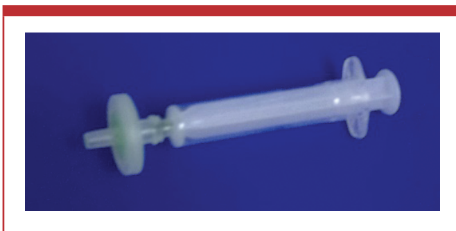
Figure 8: Syringe with filter used for injection into sampler vials (photo courtesy of NPPTL)
