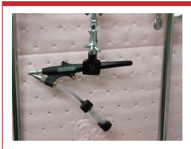
Figure 1: Airbrush sprayer used for initial investigation of contamination application (photo courtesy of NPPTL)
