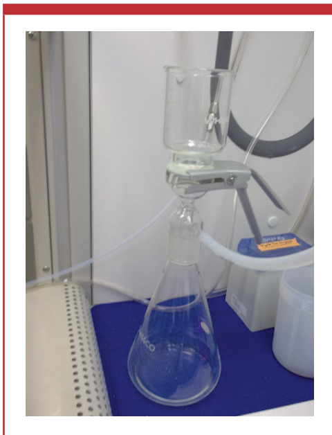
Figure 6: Filtration apparatus used in extraction of contaminated swatch (photo courtesy of NPPTL)
