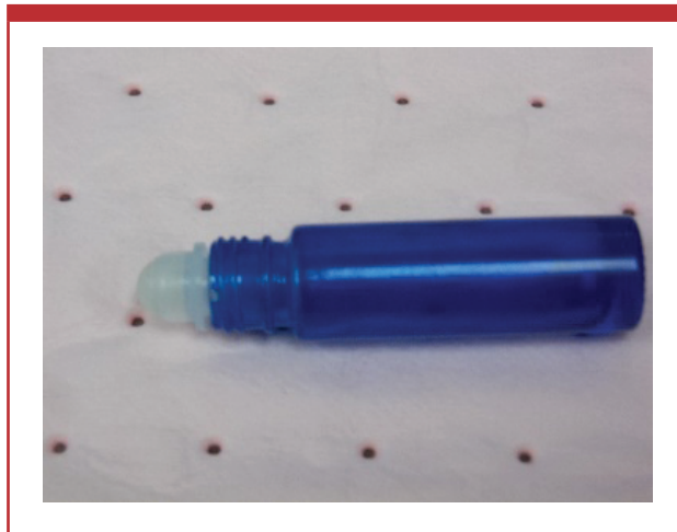
Figure 2: Rollerball applicator used as alternative contamination technique (photo courtesy of NPPTL)
