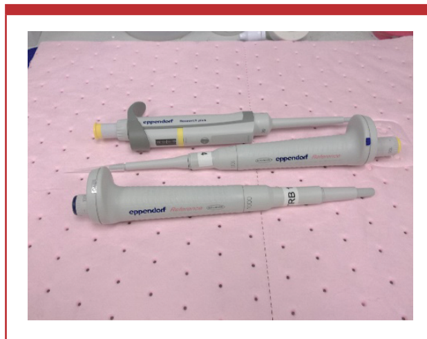
Figure 4: Pipettes used for applying contaminated solutions onto swatches (photo courtesy of NPPTL)
